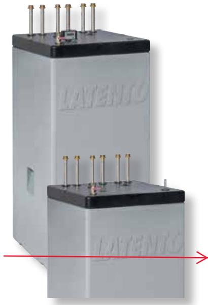
Pressure-free plastic solar storage according to DIN 4753 and DIN 4708, in particular suitable for operation with regenerative systems (for low subsequent heating performance, e. g. with heat pumps), with integrated PUR insulation, with drinking water, heating and solar heat exchange from long-wave stainless steel corrugated pipe, exterior thread connection G 1 1/4 including latent material.
