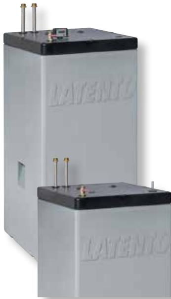
Unpressurized plastic storage tank as a buffer for recharging the boiler from different heat generating units. With integrated PUR insulation, gross volume 540 litres, with heat exchanger of long-wave stainless steel corrugated pipes for improved heat yield, external thread connector G 1¼.
