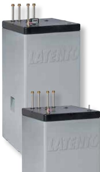
Unpressurized plastic solar storage tank for hot water generation in single and multiple-occupancy buildings. Integrated PUR insulation, gross volume 540 litres, with hot water heat exchanger and heating heat exchanger of long-wave stainless steel corrugated pipes for improved heat yield, external thread connector G 1 1/4.
