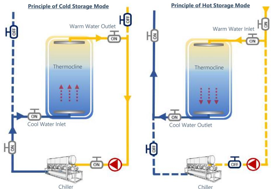
The IES unique diffuser in the thermal storage tank guarantees the laminar flow in the tanks and limits the Froude Number to be within 1. Also, the buffer plates are installed at different heights of the tank to minimize the mixing between the chilled water and the high-temperature return water. Temperature data logging system may also be equipped at different heights for purposes of performance monitoring and data collection.
