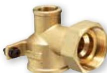
**LATENTO** connection bracket for mounting to **LATENTO** holder for connection bracket stepped (878700093), sound-proofed installation thanks to polyamidewashers on securing screws of type M 5 suitable for sanitary, heating sectors as well as solar, material: brass, polyamide, steel, annealed cast iron.
