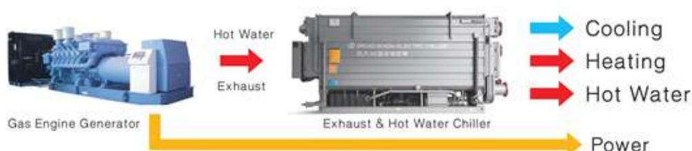
The input heat energy heats LiBr solution to 140°C and generate vapor, which is then condensed into water by cooling water. When the refrigerant water enters evaporator (in high vacuum condition), its temperature goes down immediately to 5°C and is sprayed over the evaporator tubes, to make chilled water drop down from 14°C to 7°C to make cooling. The refrigerant water absorbs heat from air conditioning system and evaporates, then is absorbed by concentrated LiBr solution from the
